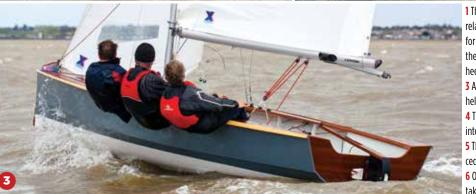
1 The height of the side deck relative to the cockpit floor makes for comfortable hiking 2 Upwind the 550 remained balanced when heeled, even when in need of a reef 3 A reef in the main would have helped upwind in the conditions 4 The wide cockpit has attracted interest from training centres 5 The 550 has a classic appeal with cedar and sycamore detailing 6 On hoisiting the spinnaker, the 550 takes off downwind like a dinghy
